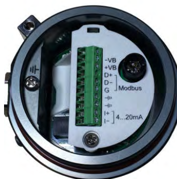
Screw terminals with signal labels inside the connection chamber
